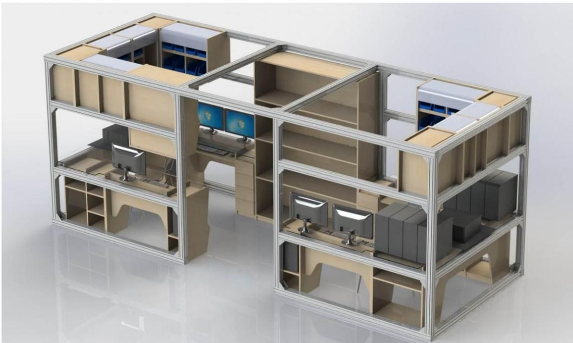
Figure 4. Computer graphic of the final 3D model of the prototype island based on the established WEEE process layout
